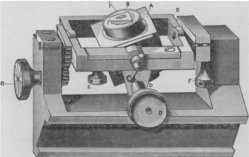
FIG. 3.—The Object-holder and Carrier.
